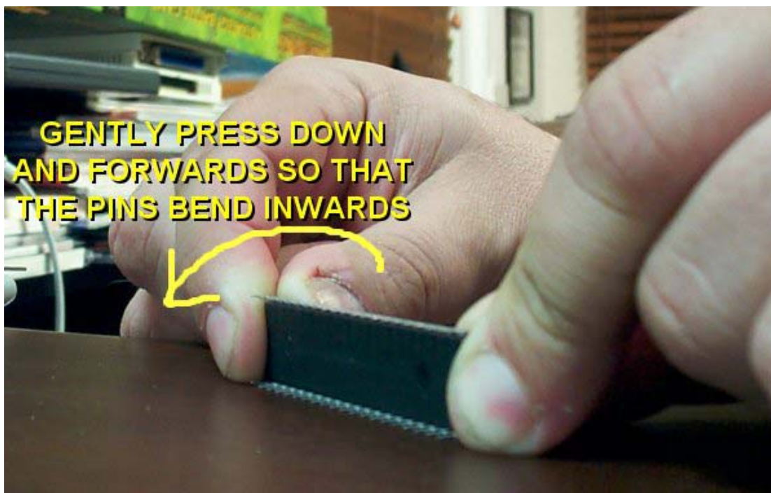
Figure 6 – using a desk and gentle pressure to bend the pins inwards
